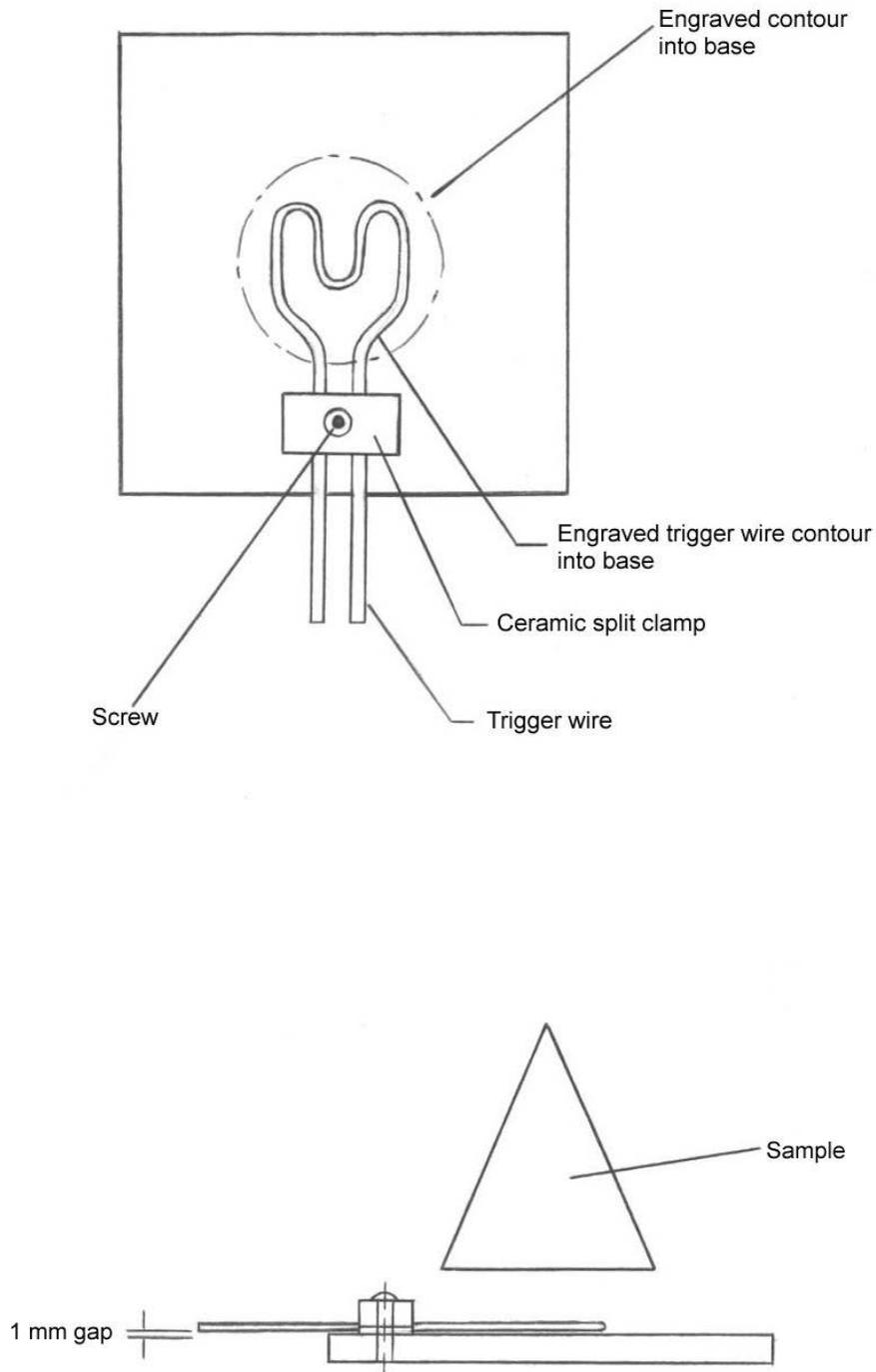
TEST METHOD FOR OXIDIZING SOLIDS
